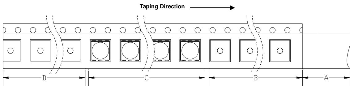
A: Top Cover Tape, 300mm; B: Leader, Empty, 200mm; C: 5500 Lamps Loaded; D: Trailer, Empty, 200mm.
